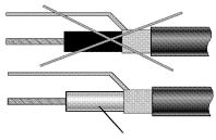
Black, semi conductive synthetic layer has to be removed completely.
